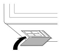
To reinstall the grease filter, insert the back of the filter, push the filter toward the back, and lift the filter up into place.
