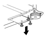
**7** Remove the bottom hinge bracket from the right side of the housing.
