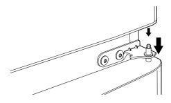
**3** Carefully snap the top hinge cover back into place over the hinge.
