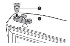
Reverse the hinge lever **9** by flipping it over. Place it on top of the bracket and tighten both down with the screw.
