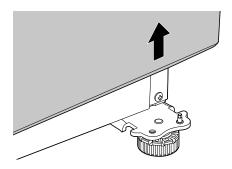
3 Loosen the 2 bolts and the Phillips head screw and remove the middle hinge bracket from the refrigerator housing. Set the parts aside.
