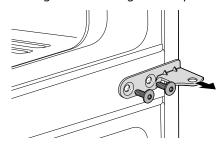
4 Using a 1/4 in. socket wrench, loosen and remove the bottom hinge pin 4 from the bottom hinge bracket 5. Remove the washer from the bottom hinge pin and set it aside.
