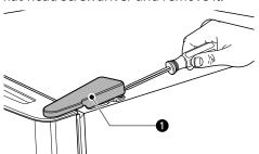
Using 10 mm or 3/8 inch socket wrench, remove the three bolts and lift the top hingeSet parts aside.
