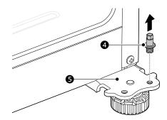
**5** Reattach the bottom hinge pin to the opposite side of the bottom hinge bracket.
