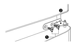
Lift up the refrigerator door slightly and remove it. Set the door aside on a nonscratching surface.
