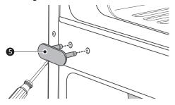
Flip the middle hinge bracket **6**. (The flange will now be on top.) Position it on the left side of the refrigerator and reattach it with two bolts and a Phillips-head screw.
