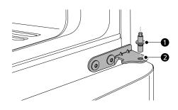
**2** Slightly lift the refrigerator door and remove it.
