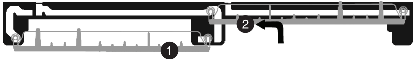
Left rack adjusted to lower position and right rack to upper position
