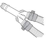
**3** Insert the end of the drain hose connector into the laundry tub or standpipe. Use the band clamps to keep it in place, if needed.
