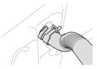
**3** Adjust the band clamp with pliers to keep the hose securely in place and prevent leaking.
